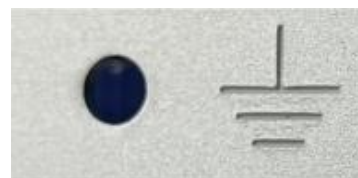
Fig. 13: detail view of equipotential bonding hole and symbol
