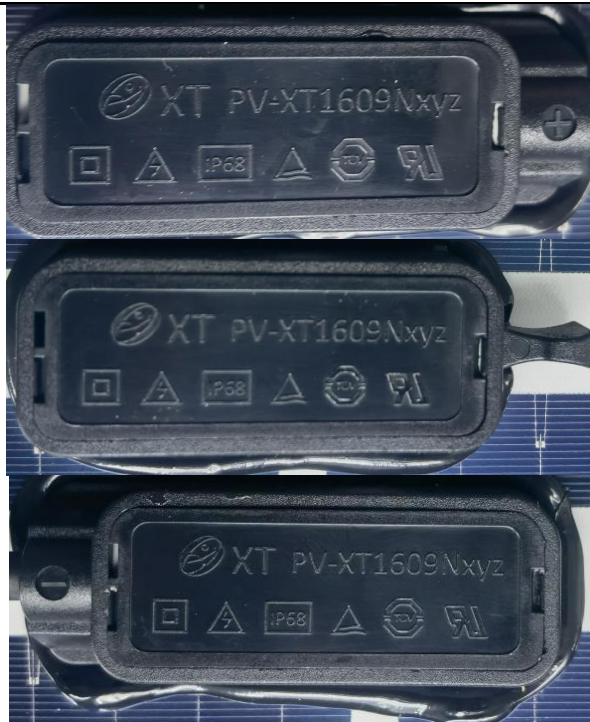
Fig. 5: detail view of closed junction box
