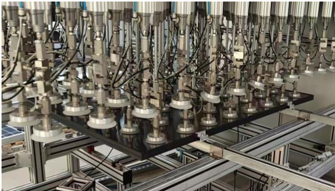
Fig. 12: view of mechanical load mounting
