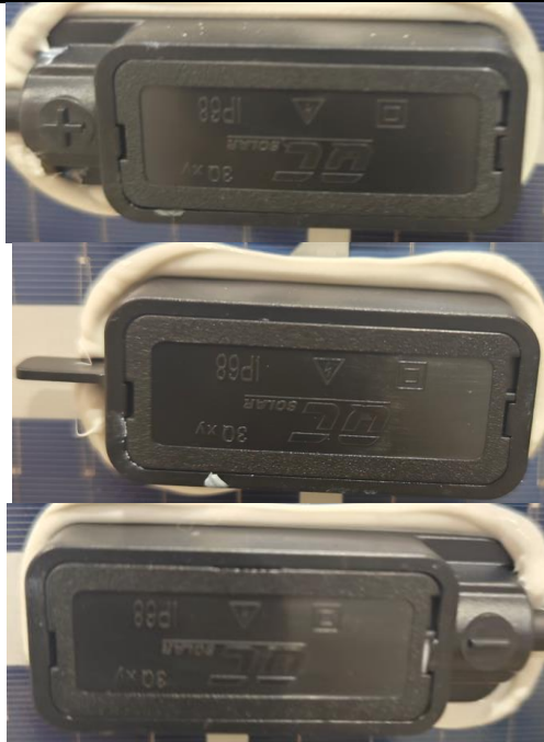
Fig. 22: detail view of closed junction box
