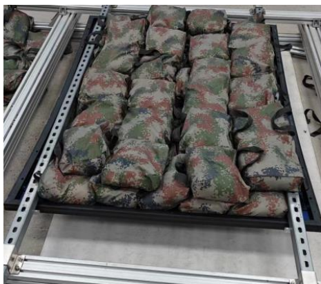
Fig. 14: view of mechanical load mounting
