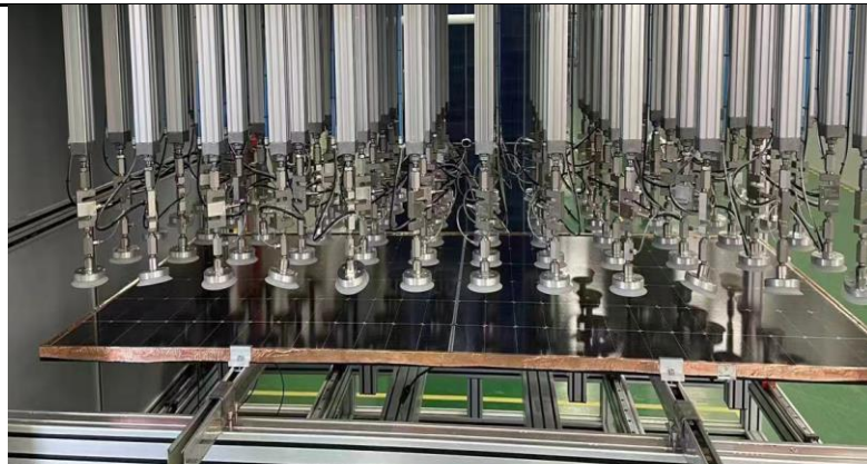
Fig. 10: view of mechanical load mounting
