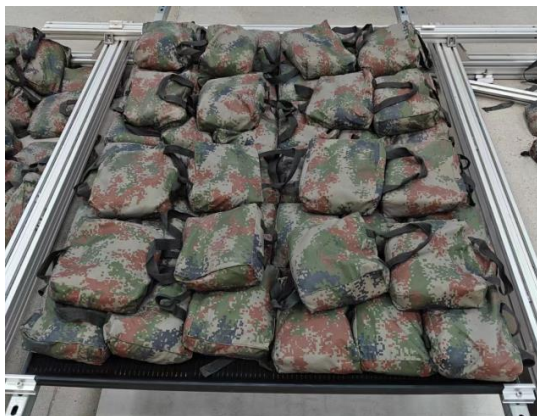
Fig. 16: view of mechanical load mounting
