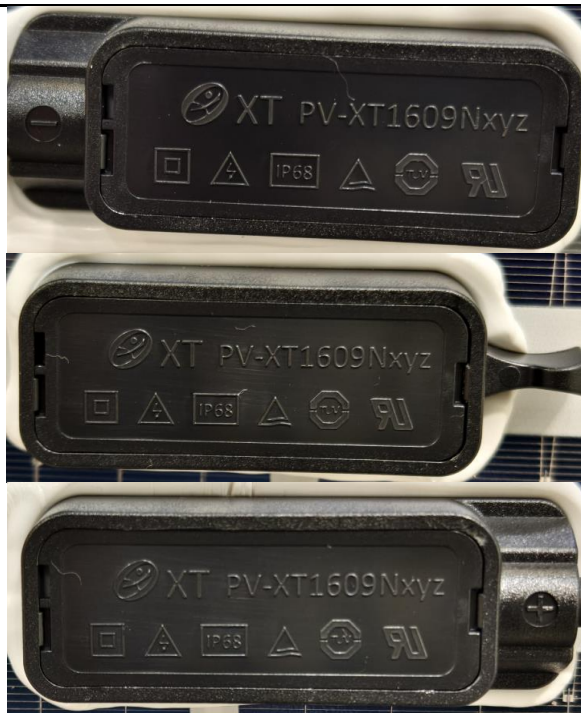
Fig. 14: detail view of closed junction box
